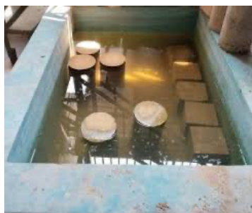
Gambar 5. Proses water curing
