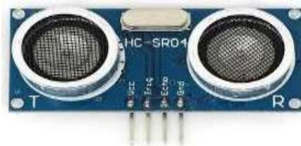
Gambar 3. Sensor Ultrasonic HC-SR04
