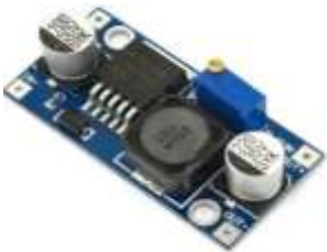
Gambar 4. Step Down LM2596
